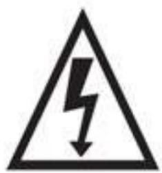
THE LIGHTNING FLASH WITH ARROWHEAD SYMBOL, WITHIN AN EQUILATERAL TRIANGLE, IS INTENDED TO ALERT THE USER TO THE PRESENCE OF UNINSULATED "DANGEROUS VOLTAGE" WITHIN THE PRODUCT'S ENCLOSURE THAT MAY BE OF A SUFFICIENT MAGNITUDE TO CONSTITUTE A RISK OF ELECTRIC SHOCK TO PERSONS.
