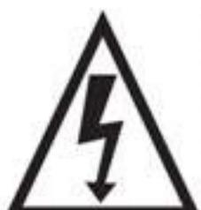
LE SYMBOLE COMPORTANT UN ECLAIR INSERE DANS UN TRIANGLE EQUILATERAL AVERTIT L'UTILISATEUR DE LA PRESENCE D'UNE HAUTE TENSION DANGEREUSE, SANS ISOLATION ELECTRIQUE. A L'INTERIEUR DE L'APPAREIL LA TENSION PEUT ETRE SUFFI-SAMMENT ELEVEE POUR PROVOQUER DES RISQUES DE CHOC.
