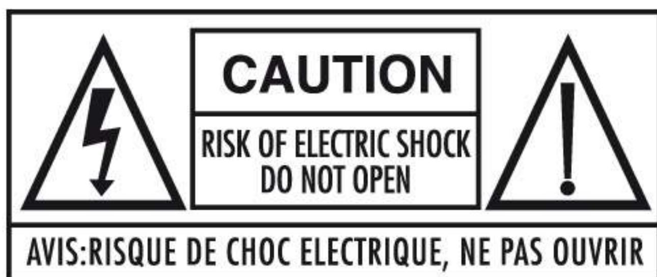
THE LIGHTENING FLASH WITH THE ARROWED SYMBOL,WITHIN AN EQUILATERAL TRIANGLE, IS INTENDED TO ALERT THE USER TO THE PRESENT OF UNINSULATED "DANGEROUS VOLTAGE" WITHIN THE PRODUCT'S ENCLOSURE THAT MAY BE OF A SUFFICIENT MAGNITUDE TO CONSTITUTE A RISK OF ELECTRIC SHOCK TO PERSONS.
