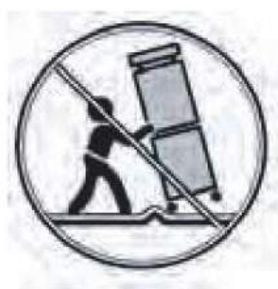
12) Use only with the cart, stand, tripod, bracket, or table specified by the manufacturer, or sold with the apparatus. When a cart is used, use caution when moving the cart/apparatus combination to avoid injury from tip-over.
