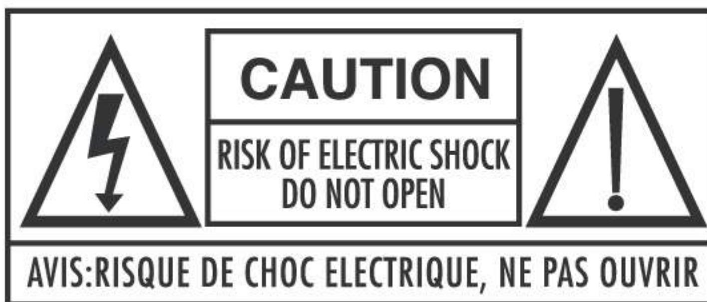
THE LIGHTNING FLASH WITH ARROWHEAD SYMBOL, WITHIN AN EQUILATERAL TRIANGLE, IS INTENDED TO ALERT THE USER TO THE PRESENCE OF UNINSULATED "DANGEROUS VOLTAGE" WITHIN THE PRODUCT'S ENCLOSURE THAT MAY BE OF A SUFFICIENT MAGNITUDE TO CONSTITUTE A RISK OF ELECTRIC SHOCK TO PERSONS.
