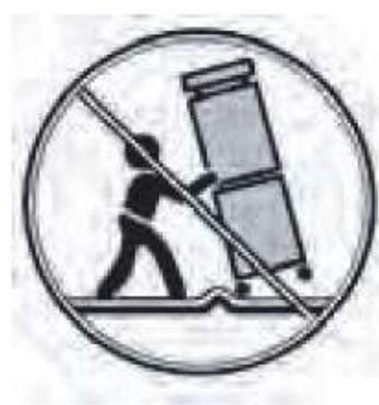
12) Use only with the cart, stand, tripod, braket, or table specified by the manufacturer, or sold with the apparatus. When a cart is used, use caution when moving the cart/apparatus combination to avoid injury from tip-over.
